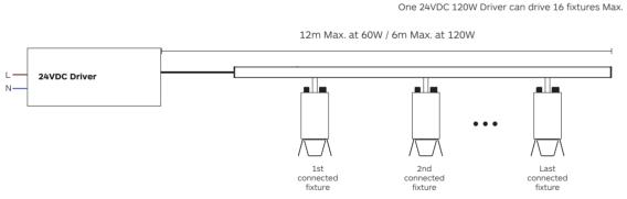
Power supply for Zero Low Voltage Surface
